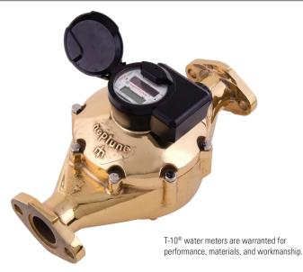
Every T-10® water meter meets or exceeds the latest AWWA C700 Standard. Its nutating disc, positive displacement principle has been time-proven for accuracy and dependability since 1892, ensuring maximum utility revenue.
